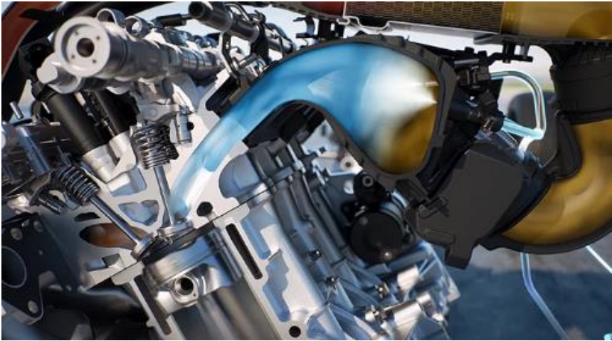
Figure 5: BMW M4 GTS water-injection system. (BMW, 2015)
