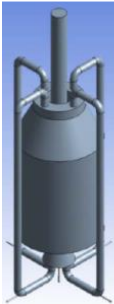
Figure 1: Bluff-body MILD combustor. ( Noor et al, 2013 )
