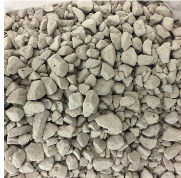
Figure 10. Mortar after LA testing
