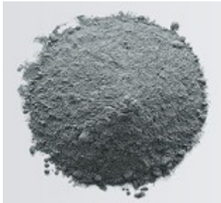
Figure 2: Fly ashes. ( http://www.silotransport.cz/en/fly-ash )
