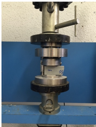
Figure 8: Compression test UNE-196-1. DIOPMA Laboratory of Materials
