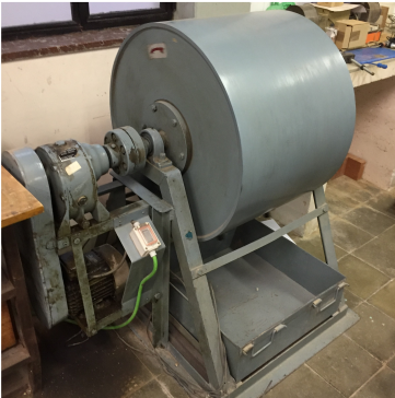
Figure 9: Abrasive testing machine LA
