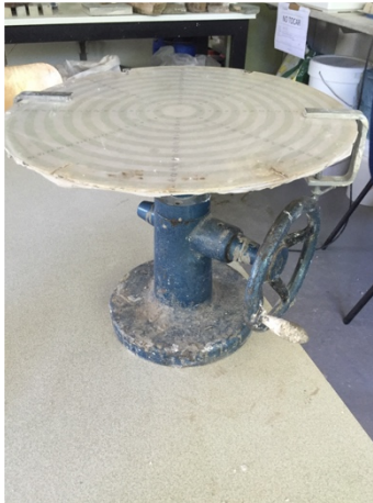
Figure 6: Shaking table, Material Laboratory UPC ETSEB
