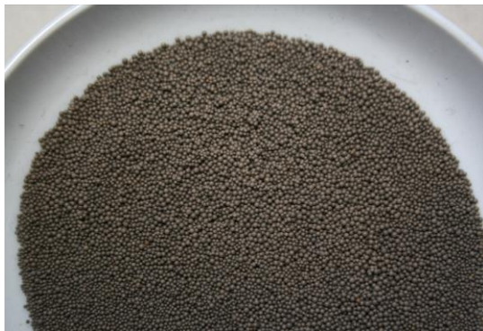
Figure 5. Example of a dried ion-exchange resin.
