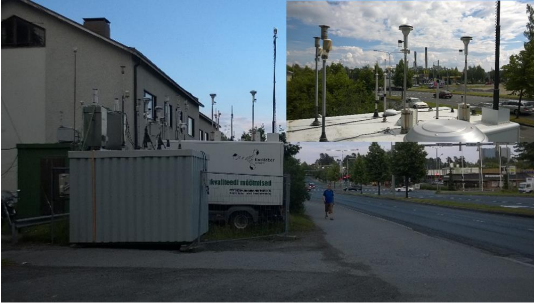
Figure 3.3. The air quality measurement site at Tasavallankatu in the city of Kuopio. The measurement van and the cabin are shown in front. The green cabin in behind is for the air quality measurement station.
