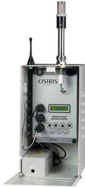
Figure 2.7. Osiris optical dust monitor
