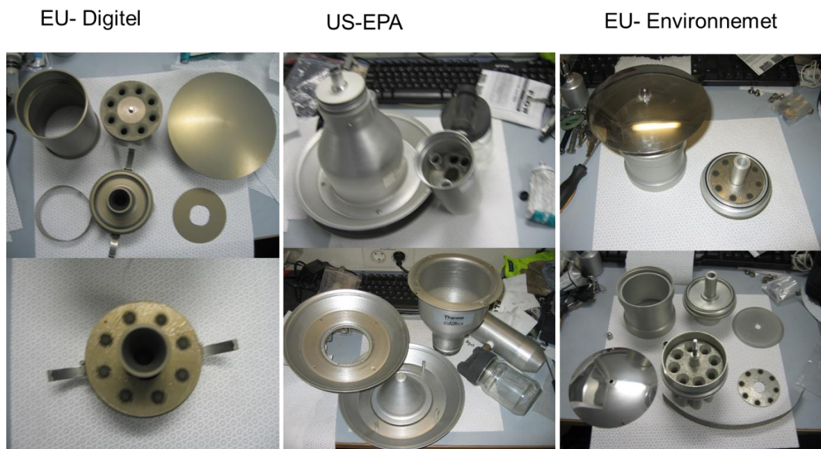
Figure 2.13. Size selective inlets used for CM: EU-Digital (FH 62 I-R, SHARP), US-EPA (BAM) and EU-Environnement (MP101).
