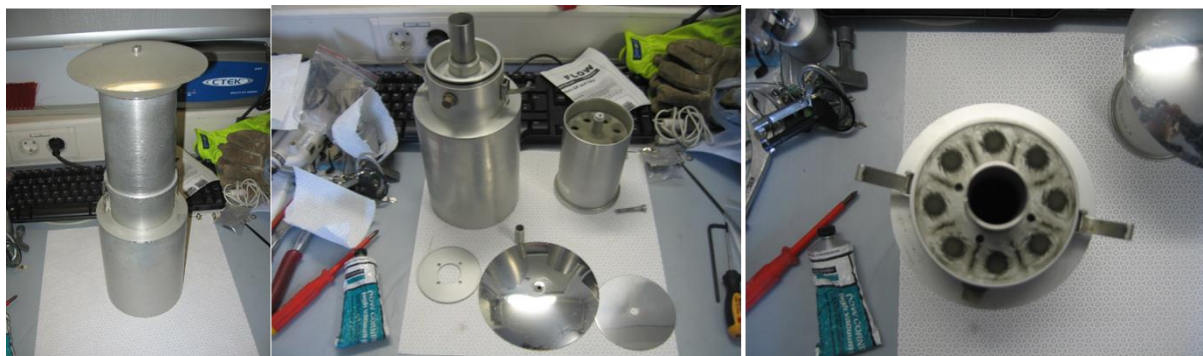
Figure 2.12. The sampling inlet for the reference method used in Leckel: Complete (in the left), separated (in the middle) and the impactor plate (in the right).
