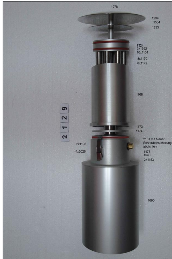
Figure 2.3: The sampling inlet of the sequential sampler SEQ47/50.
