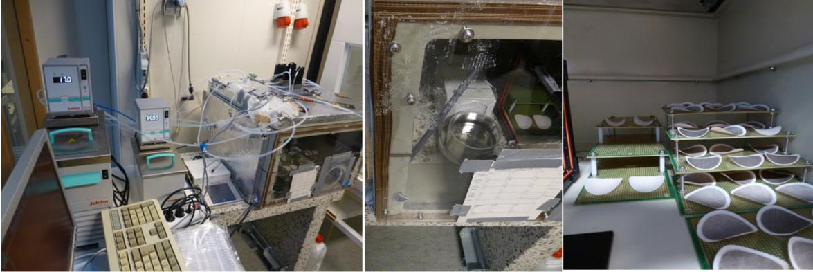
Figure 3.6: The weighing box for the filters and the control units for conditioning of temperature and humidity (on the left) with the balance (on the top middle) and the filter tray (on the right).
