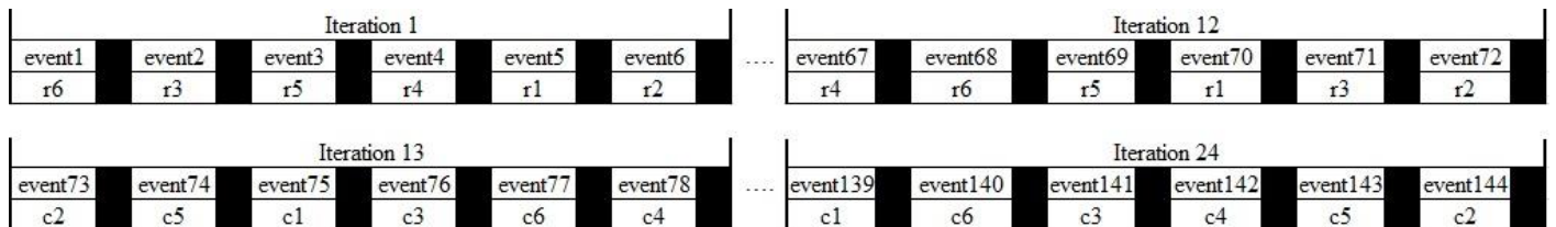
Fig. 3. The flashing technique for the RCP or EP. (r: row or row edge point, c: column or column edge point).
