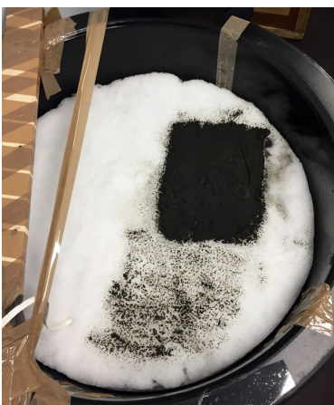
Fig. 5 During the Ash in Container (AiC-2015) experiment, two different amounts of ash were deposited on snow over of ice. Bottom 15 g ( 166 \text{ g m}^{-2} ) and top 425 g ( 4722 \text{ g m}^{-2} , 15 mm layer thickness) of 1 \phi ash
