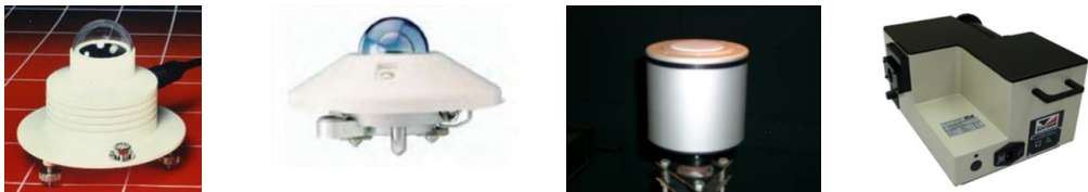
Figure 3.1. Incoming and outgoing solar irradiance data measured by broadband (type SL-501 and CM-14), multifilterband (type NILU-UV) and spectral (type Bentham) radiometers were used in PAPER I-II.
