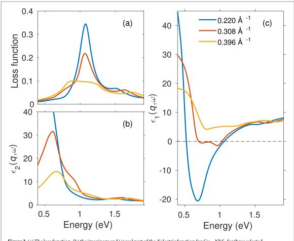
Figure 2. (a) The loss function, (b) the imaginary and (c) real part of the dielectric function for  $Cu_{0.2}NbS_2$  for three selected momentum transfers.
