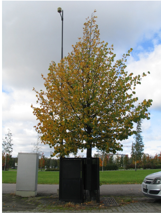
Figure 4. One of the measuring points at the Tilia site, seen in autumn 2011. Datalogger box on the left along with the temperature and PAR radiation measuring pole. The tree adjacent to the datalogger box was instrumented with sap flow sensors; the black plastic radiation shield can be seen attached to the inside of the trunk guard.
