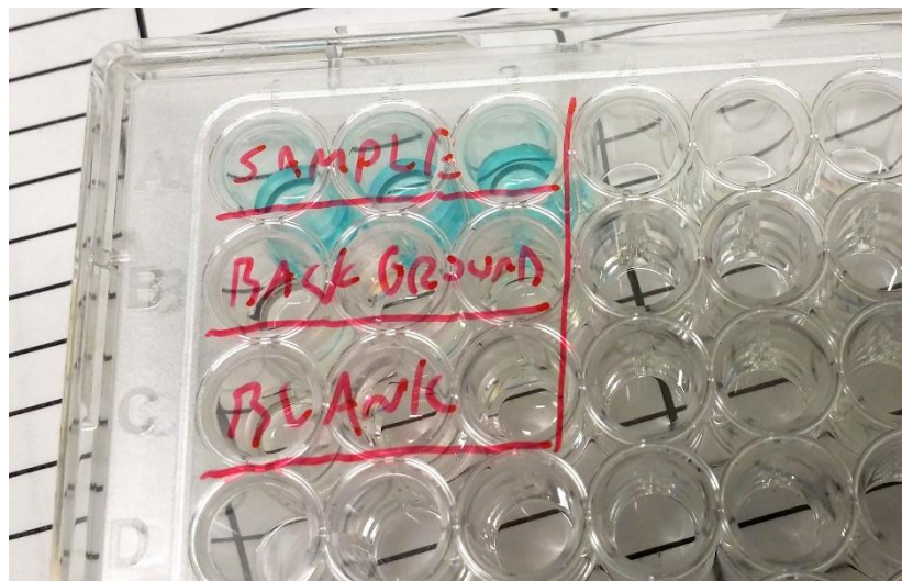
Figure 12. A close-up photograph from a 96-microtiter well plate after carrying out the BrdU ELISA protocol in whole. The strong colouration is produced by metabolically active bacteria from an exponential phase culture.
