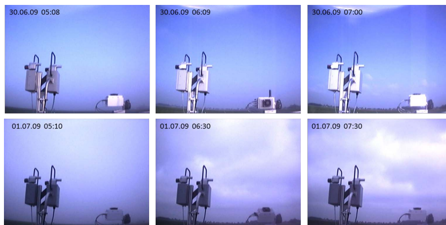
Figure 8. Webcam images from the mornings of 30 June and 1 July 2009, when foggy conditions prevailed. The webcam pointed to the viewing direction of the MAX-DOAS Instruments (north-east). The devices in the foreground are the telescopes of the Heidelberg group.
