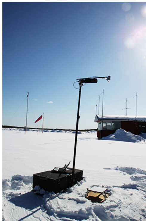
Figure 2. FIGIFIGO at the SoS test site at Sodankylä Airport. A clean snow sample has been measured, and the last reference measurement of the white Spectralon® panel is being taken. Deep and soft snow complicated the usability of FIGIFIGO. While the movements in the snow left significant traces, the target area under the instrument footprint was carefully kept untouched during the measurement.
