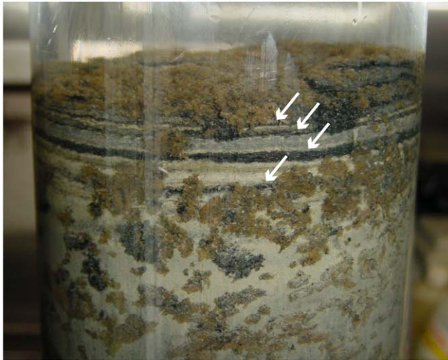
Figure 7. A sediment core from the western Gulf of Finland. The core was sampled from the station JML. Black layers (white arrows) indicate presence of ferrosulphides which are formed via reaction of ferro-iron and sulphite, produced by sulphate reducing bacteria. doi:10.1371/journal.pone.0021555.g007
