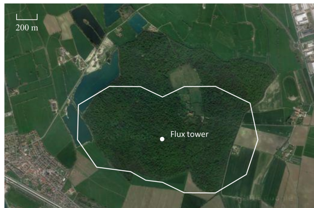
Figure 2. Satellite image (map data © Google 2016) of the field site showing the flux tower and footprint containing 80% of the flux measured during the campaign (13 June–11 July 2012).
