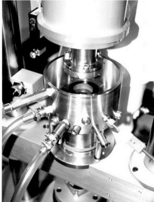
Figure 25. TE-92 Plint tribometer for the sealing tests of HFCVD diamond-coated \text{Si}_3\text{N}_4 mechanical seal faces.
