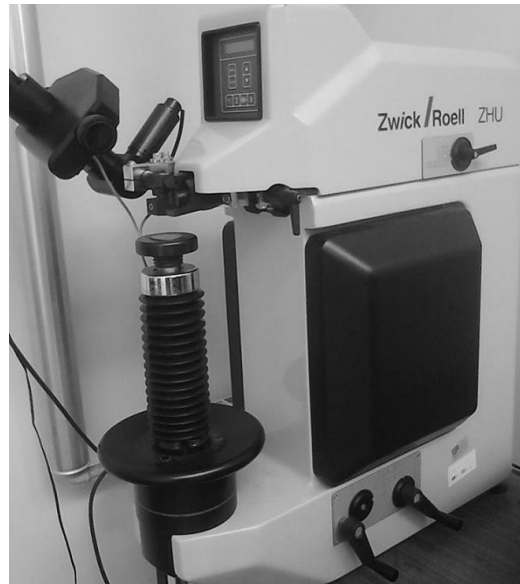
Figure 19. Apparatus for hardness and fracture toughness of sintered Si 3 N 4 ceramic substrates.
