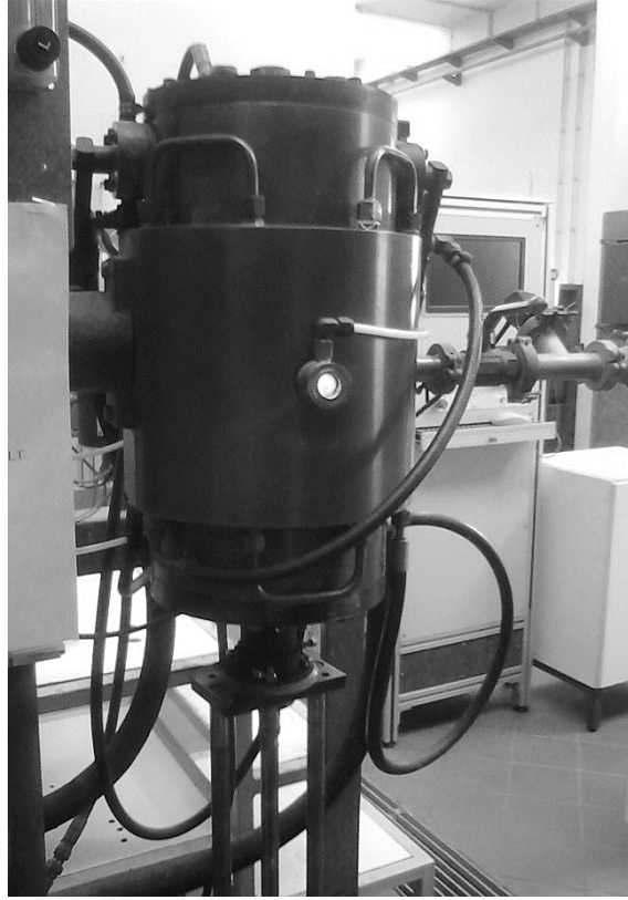
Figure 18. Graphite furnace for sintering of \text{Si}_3\text{N}_4 ceramic substrates in \text{N}_2 atmosphere used in the work.
