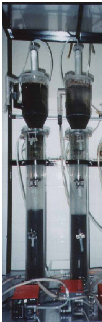
Figure 1. Laboratory-scale UASB reactors used in this work.
