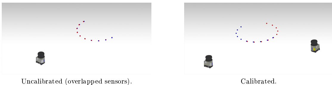
Figure 3.2: Difference between uncalibrated and calibrated sensors.
