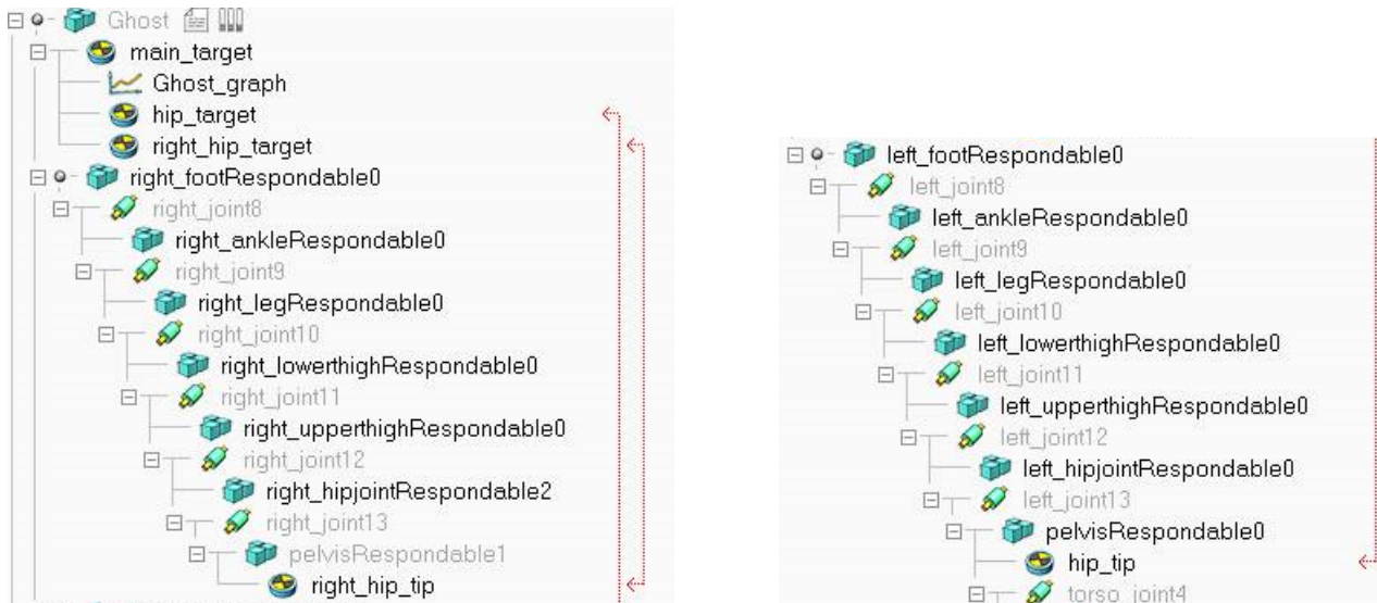
Figure 4.2: Hierarchies for the lower body of GHOST
