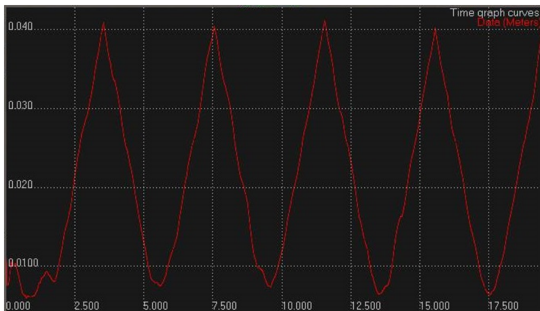
Figure 4.4: Display of the calculated distance on a full cycle while PHUA lays still
