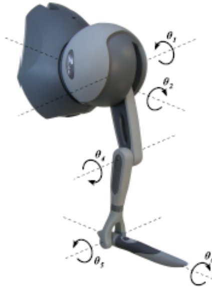
Figure 5.2: Vertical Configuration for the Phantom OMNI.
