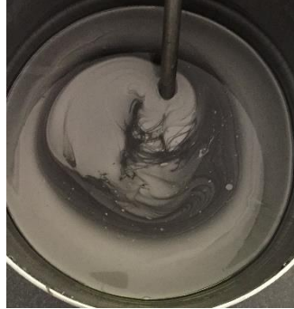
Figure 3.2 Original chrome paint, without diluent, mixed for 5 minutes.
