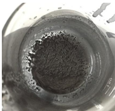
Figure 3.14 Sediments of CNTs and/or polymeric material of the stick on the bottom of the jar.
