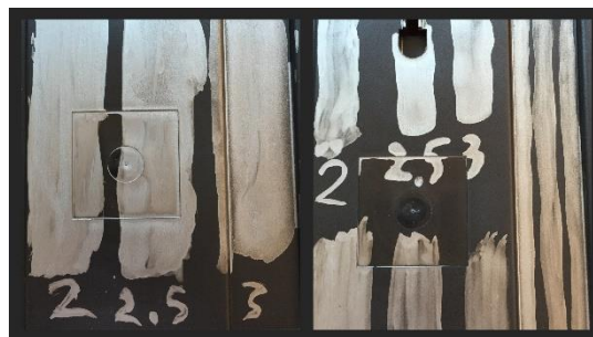
Figure 3.20 First application of diluted paints using a common brush: 2 indicates the paint diluted to 200%, 2.5 to 250% and 3 to 300%.
