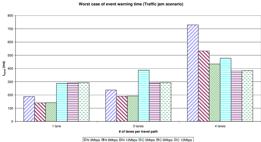
Fig. 5.15 - Worst case of event warning time per number of lanes (traffic jam)
