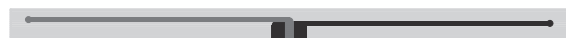
Fig. 4. Physical layout of the node's antenna (on a 1:2 scale). The antenna consists of a pair of radiating arms printed on a rectangular-shaped substrate board (one arm printed on each side).
