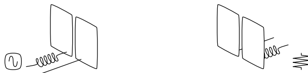
Figure 4.13: Graphical illustration of resonant electrical coupling proposed based on the circuit model shown in figure 4.1.
