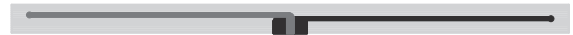
Fig. 4. Physical layout of the proposed antenna (on a 1:2 scale), in which the large rectangular area corresponds to a substrate board and the copper shapes represent a pair of radiating structures, printed on opposite sides of the board.
