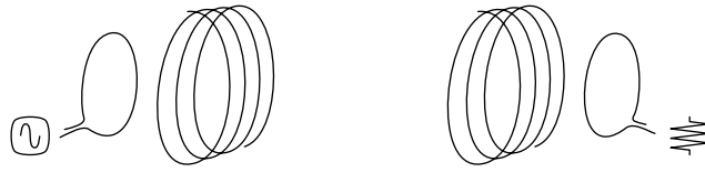
Figure 1.2: Graphical illustration of strongly coupled magnetic resonances, consisting of two single-turn loops and two helical coils.
