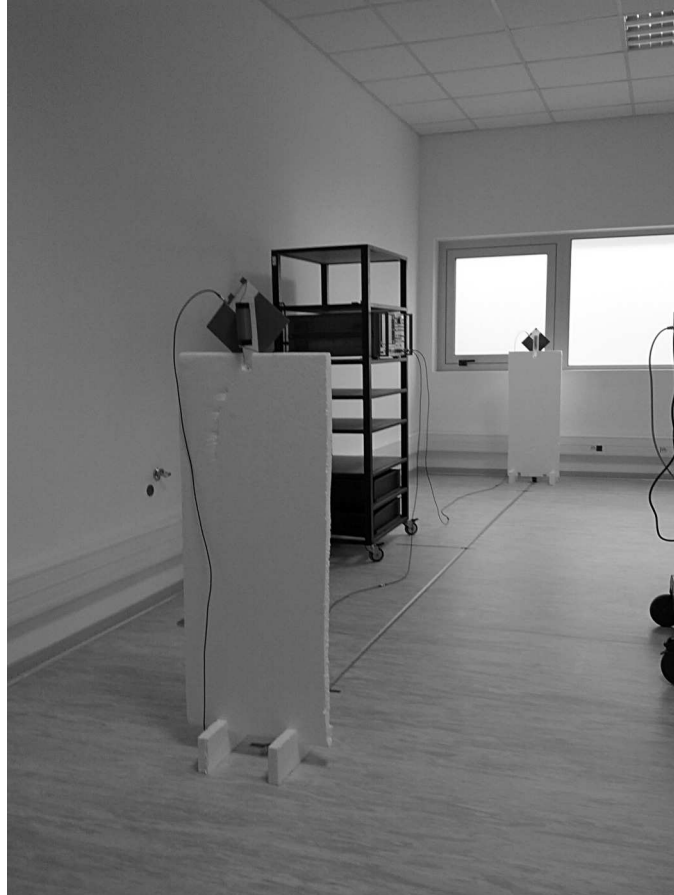
Figure 5.2: Experimental setup for measuring the scattering parameters of the prototype shown in figure 5.1.
