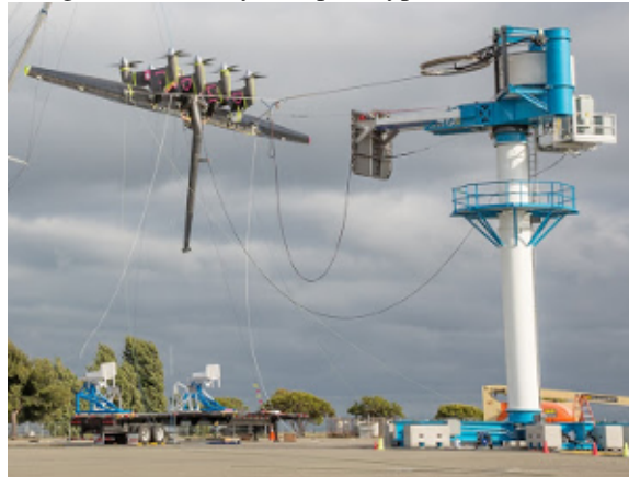
Figure 10 – Drag-mode AWE system prototype with 600kW of rated power.
