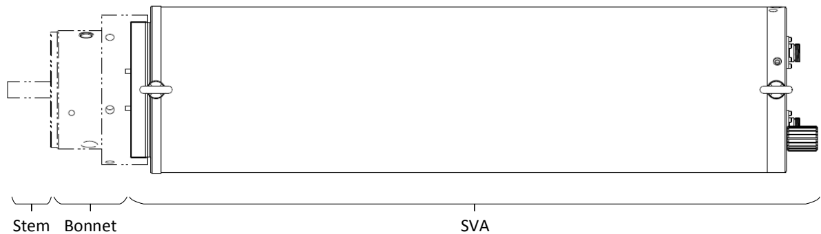
Figure 2.2: Current external mechanical design of the SVA [40]
