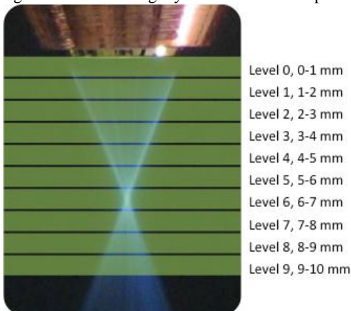
Figure 37 – Recording layers' scheme of the powder jet.
