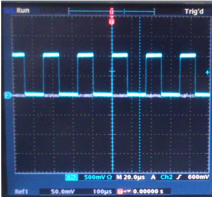
Figure 75 – The output of one of device which is accurate, precise and stable, in horizontal scale each division correspond to 20 \mu s and in vertical scale each division correspond to 500 mV, V_{dd} = 1 V , T = 20 ^\circ C .
