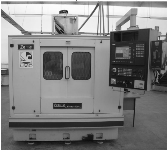
Figure 20 – Universal cylindrical CNC grinding machine (Zema Zselics Ltda Pratika Flexa 600-L).
