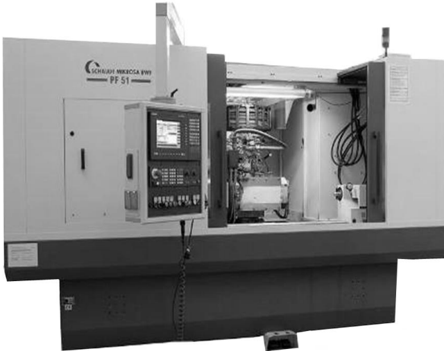
Figure 22 – Universal cylindrical CNC grinding machine (Schaudt Mikrosa BWF, PF 51).
