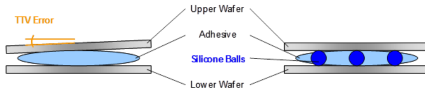
Figure 4.26: TTV avoiding function of specialized adhesives
