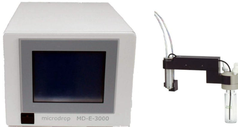
Figure 2.1: Standard micro dispensing system with touchscreen [12]
