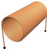
$$v(t)_{bobina} = -\mu_0 NS \frac{dH}{dt} \quad \text{Eq. 2.1}$$
