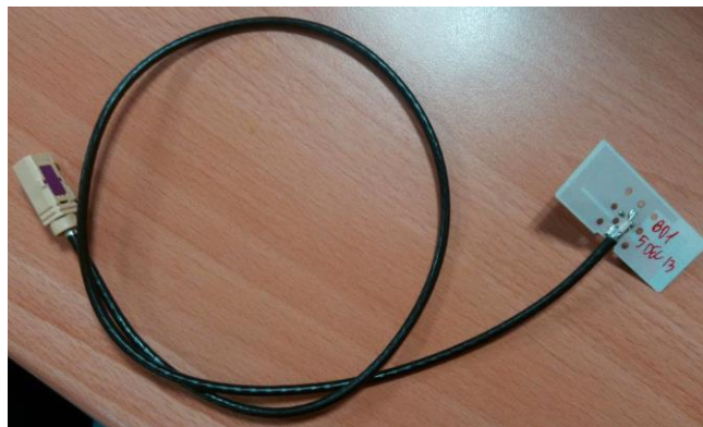
Figure 9: Wi-Fi antenna for vehicles Source: Source: Andoni Amurrio & Julio Arellano PAWS Practica 3
