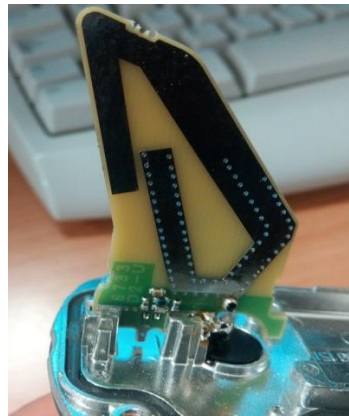
Figure 5: "Shark fin" antenna for mobile communications on board Source: Andoni Amurrio & Julio Arellano PAWS Practica 3
