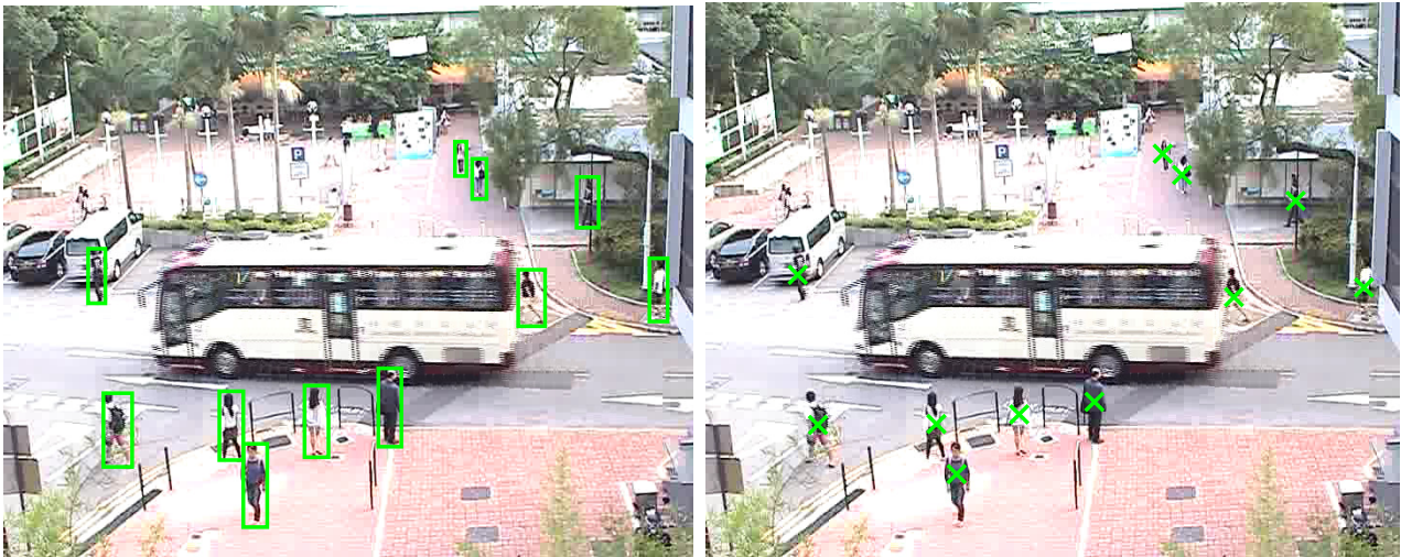
Figure 1: Strong versus weak annotation (best viewed in colour). On the left is the standard way of annotating pedestrians for training a pedestrian detector. On the right is the weak supervision (only approximate centres of pedestrians) required by our proposed algorithm. Note that pedestrians are of different sizes in the video due to projective distortion and hence our algorithm has to cope with both noisy locations and unknown scales. Weak supervision on the right is much faster and easier for a human annotator than the strong supervision on the left. Images shown are from the CUHK Square dataset [14].
