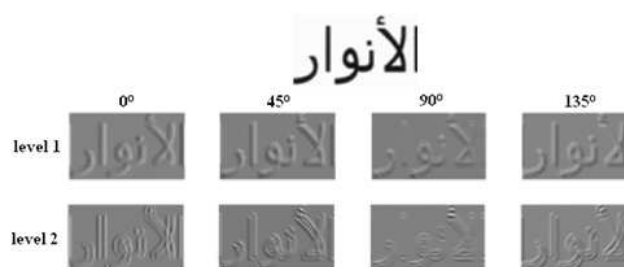
Figure 2: Decomposition with 2 levels and 4 orientations of a printed Arabic word
