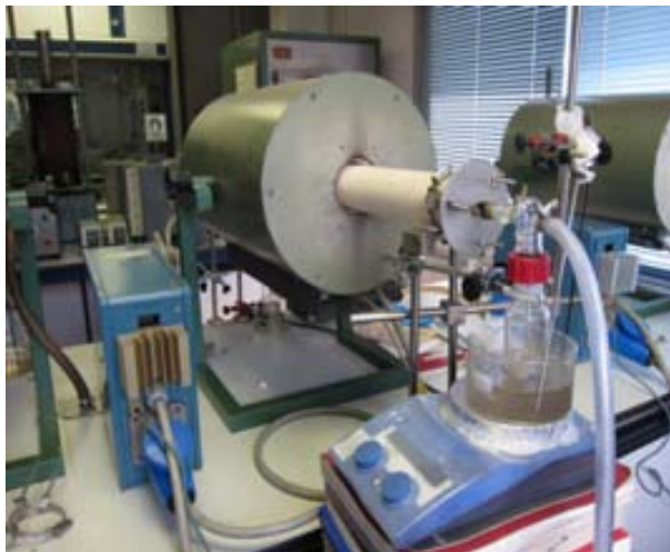
Figure 3.1. Photograph of the purification set-up. A bubbler filled with distilled water is placed on top of a heating plate and attached to a horizontal tubular furnace
