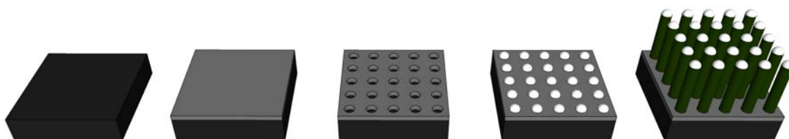
Figure 41: Process flow for hybrid selective area and self-catalytic MOCVD growth method for GaP nanowire arrays, starting with a silicon wafer, depositing a \text{SiN}_x mask layer via PECVD, patterning the mask layer using e-beam and a pseudo-Bosch RIE etch, nucleating Ga droplets in situ , and finally, growing the nanowires.
