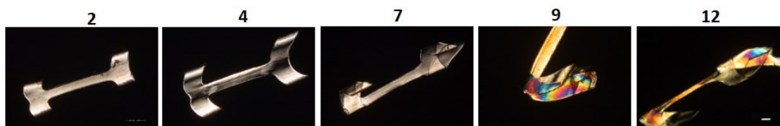
Figure 2.10: Polarized light micrographs of 10-13 \mu\text{m} thick sections acquired in a Zeiss Universal microscope through crossed linear polarizers equipped with a Canon EOS DS30 camera. The thin sections were cut from YW crests (Fig. 2.13, Methods) in the radial direction. The smallest number corresponds to the section closest to the outer diameter of the scaffold subassembly. The onset of curling is about 70 \mu\text{m} and the onset of higher retardance is about 90 \mu\text{m} from the outer surface of the as-cut subassembly. Scale bar is 100 \mu\text{m} .
