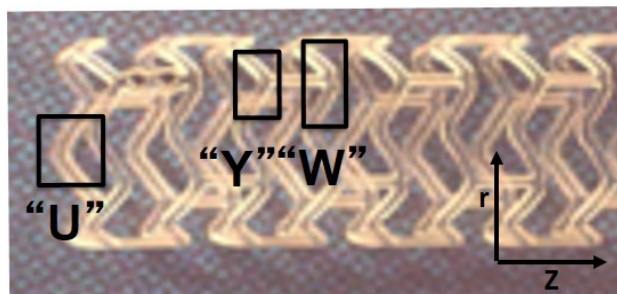
Figure 2.12 Image of an as-cut sub-assembly with boxes indicating the W, Y, and U struts.
