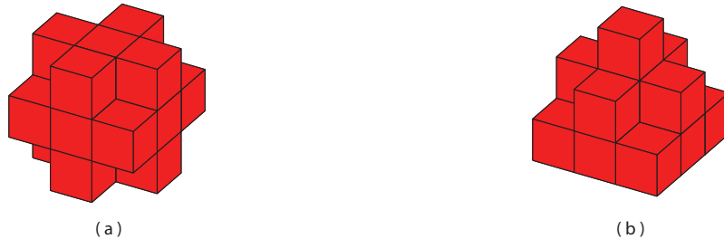
Figure 2.2: Cells used in the least square polynomial fit in 3D: a) 19 cells centered on the point of interest (non-wall), b) pyramid shaped collection of cells with the point of interest in the middle of the base (wall).
