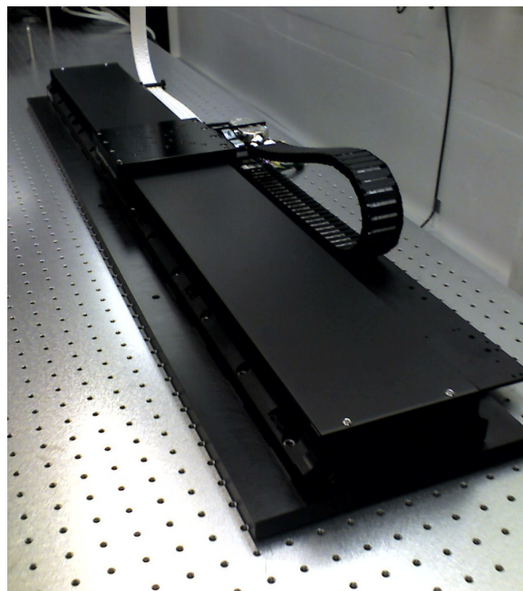
(b) A longer-range delay line offering \sim 1 m of travel and room for a quadruple pass of the light beam.
