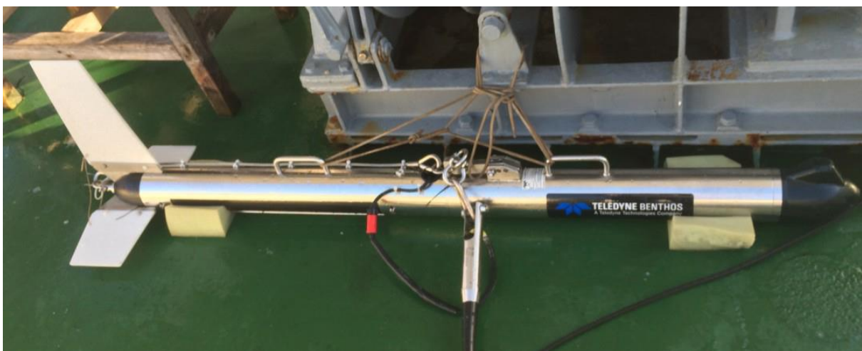
Figure 2: The employed Sidescan Sonar Teledyne Benthos, SIS-1624
