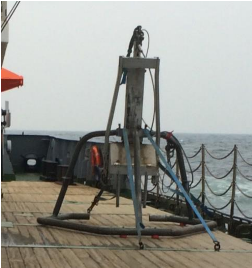
Figure 3: The employed giant box corer (box not installed) during the cruise POS505.
