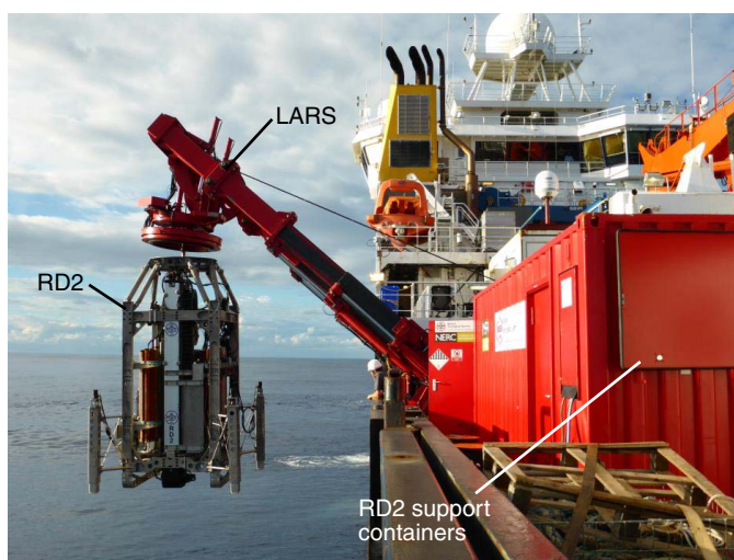
Figure F5. The BGS RD2 seabed drill deployed by its own LARS over the starboard side of the RRS James Cook , Expedition 357. Image courtesy of Dave Smith.
