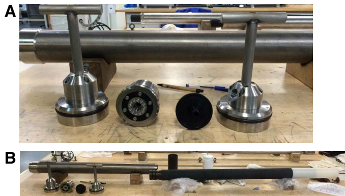
Figure F20. Component parts of the downhole plug system used by the RD2 and MeBo drills, Expedition 357. A. Downhole plug caps can be removed to allow full access to the borehole or enable borehole fluid sampling by an ROV through a valve in the cap. B. Two additional units of the borehole plug consisting of a modified drill rod with a ball valve (leftmost end of image); another section with the swellable packer material (rightmost end of image) to achieve a sidewall seal, closing the borehole to allow fluid equilibration following coring operations; and a nylon shoe.
