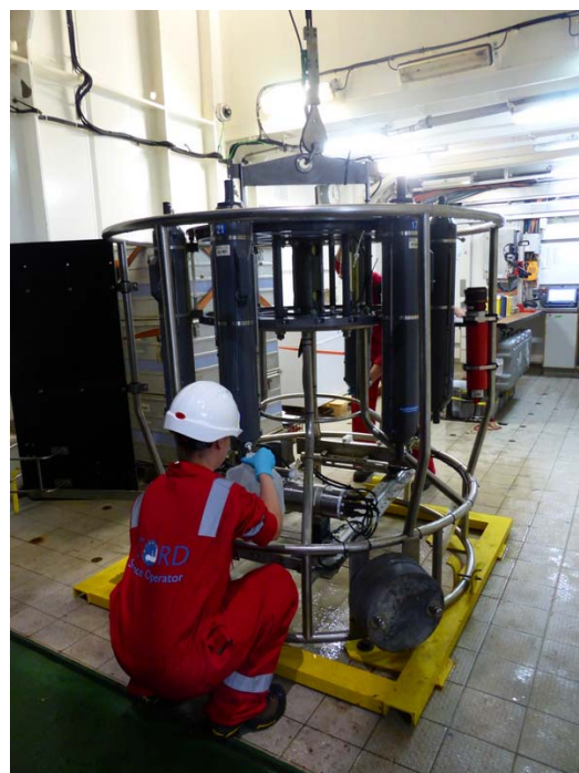
Figure F7. CTD rosette, RRS James Cook , Expedition 357. Image courtesy of Carol Cotterill.
