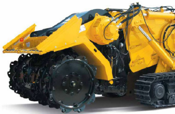
Fig. 8. Onshore road miner tools for cutting coal [13]
