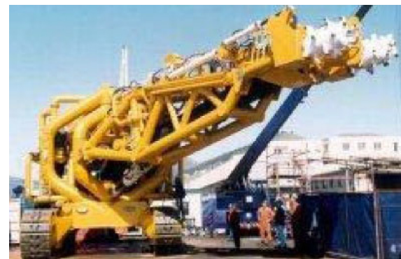
Fig. 5. 250 t Diamond Mining Machine with slewing arm [13]
