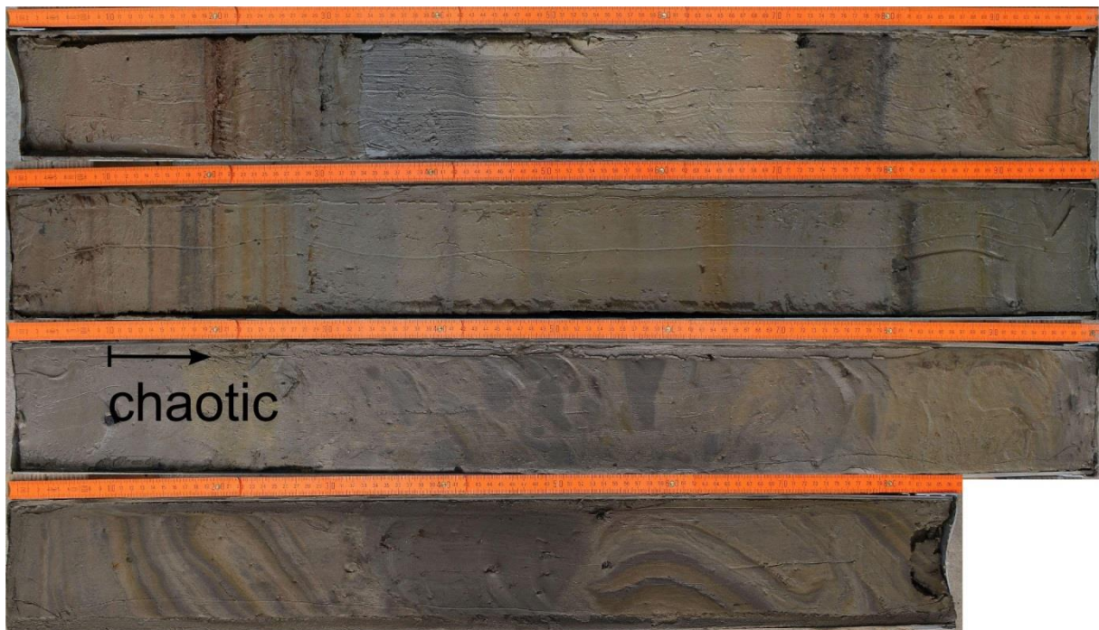
Figure 2.S2: Photograph of gravity core 606, every part of one meter length. The upper layer (0 to 210 cm) are well stratified, underneath there is chaotic sediments that we interpret as slide deposits.
