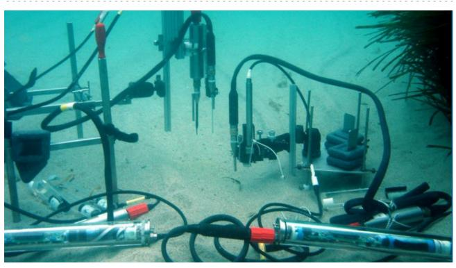
State-of-the-art sensors measure the amount of CO2 leaked from the ocean floor in the Mediterranean Sea, and similar ones are being used in the North Sea. Image credit: M.Weber/HYDRA
