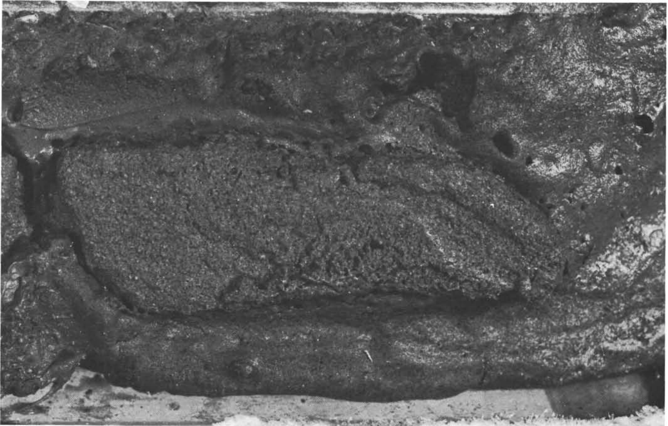
Figure 11. Gas hydrate (Sample 498A-15-2, 110–125 cm) during decomposition. (This photograph was taken less than 5 min. after the sample was brought aboard the Challenger . The hydrate is contained in a volcanic ash; the central part is solid, whereas the outer parts are a bubbling fluid.)
