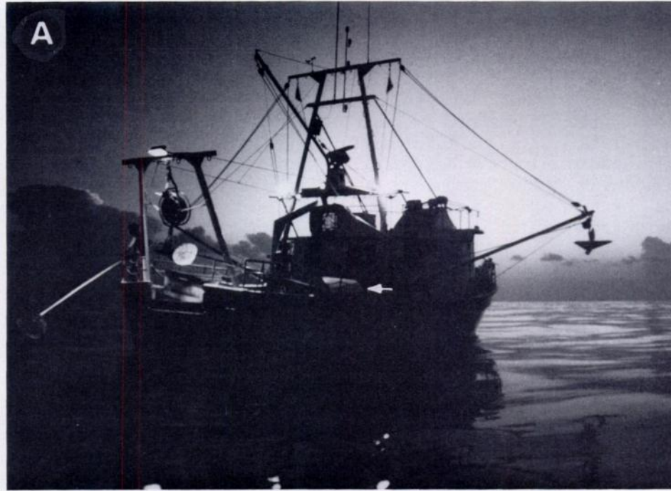
FIGURE 1. Capture and transport. A. R/V ERIN LEDDY-JONES nightlighting for Loligo plei off the coast of Galveston, Texas in 17 m of water. Note the 1000-watt quartz-iodide lamp on the A-frame and two 500-watt quartz-iodide lamps amidships that are used to attract squids. Squids are dipnetted on board (left) and placed in a transport container (arrow). B. Three types of transport containers: VT is the vertical tank; HCT is the horizontal cylindrical tank; RHT is the rectangular horizontal tank. The tanks and squids are all drawn to the same scale. The squids equal the approximate size of 200 mm mantle length. Water flow is indicated by arrows. In the RHT, (A) is the removable partition that is replaced when approximately 15 adult Loligo spp. are put in the tank. The tank top (B) is then secured with stainless steel bolts (C) that force a rubber gasket (D) against the top edge of the tank, producing a water-tight seal. Another 15 squids are placed in the upper compartment through the chimney (E). When water quality is good, sea water is continually pumped into the base of the tank through (F) and allowed to overflow from the chimney. When water quality deteriorates near shore, the tank water is circulated by a submersible pump (G) that pushes the water through an exterior filter (H) and back into the tank. Pure oxygen or air may be added through a valve (I).
