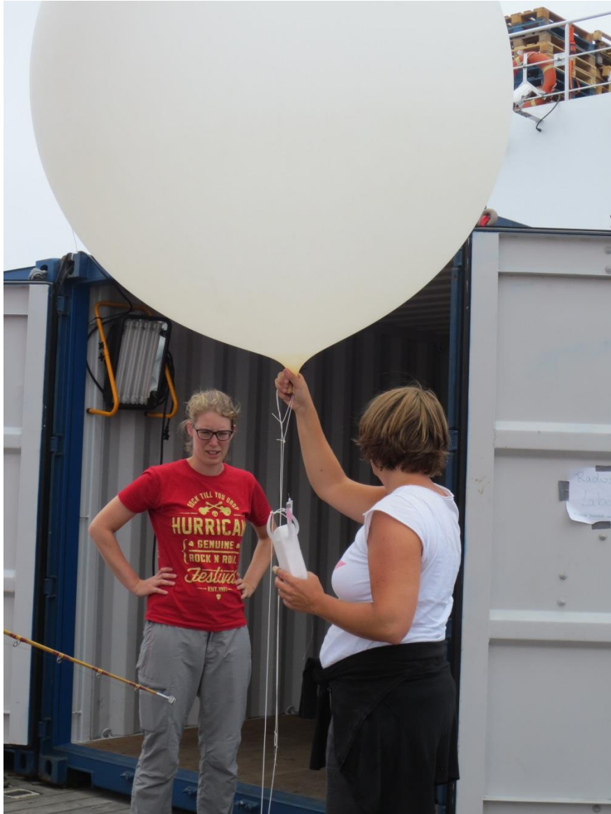
Figure 7.9.1. Preparation to launch a radiosonde from the aft deck of R/V Sonne.
