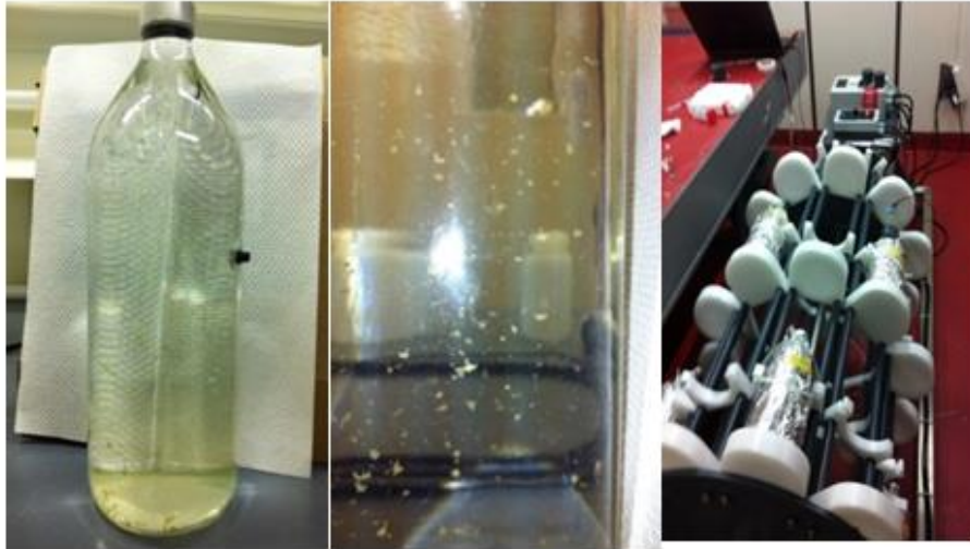
Figure 7.16.2. Incubation bottle (left) showing collected particles (middle) and rotating plankton wheel (right).
