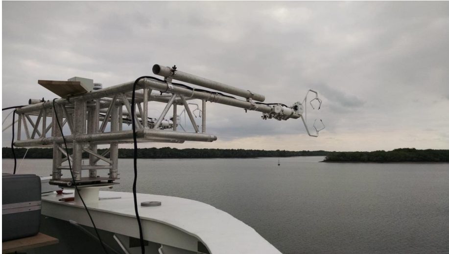
Figure 7.8.1. Eddy covariance mast on the bow of R/V Sonne in the port of Guayaquil.
