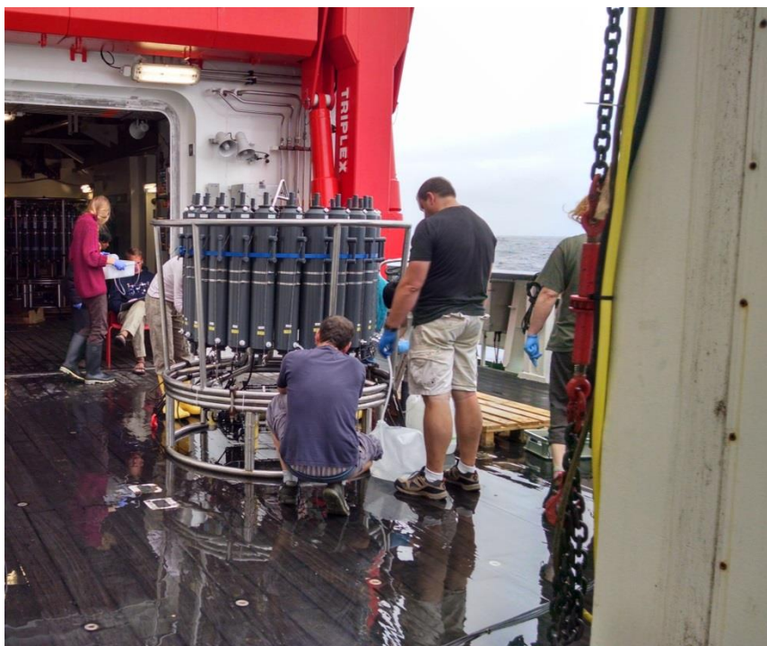
Figure 7.11.1. Sampling the Niskin bottles of the CTD rosette.
