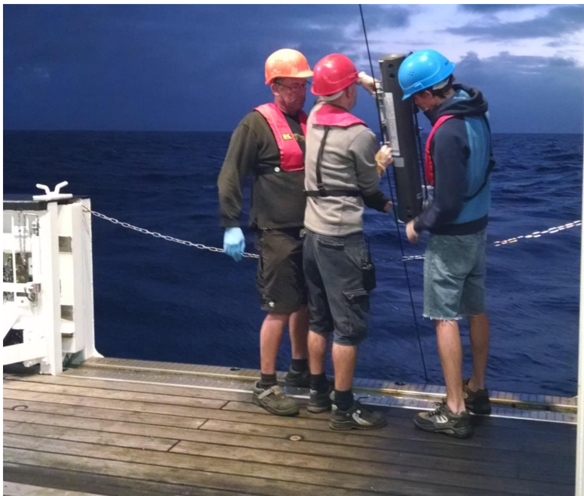
Figure 7.6.1. Deployment of a GoFlo bottle at the Kevlar wire.
