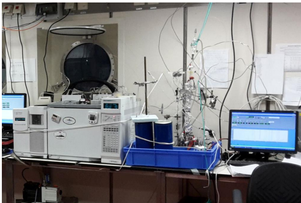
Figure 7.5.1. Halocarbon GC-MS system on board ASTRA-OMZ SO243.
