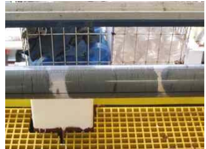
Image 2: Voids in core recovery.
