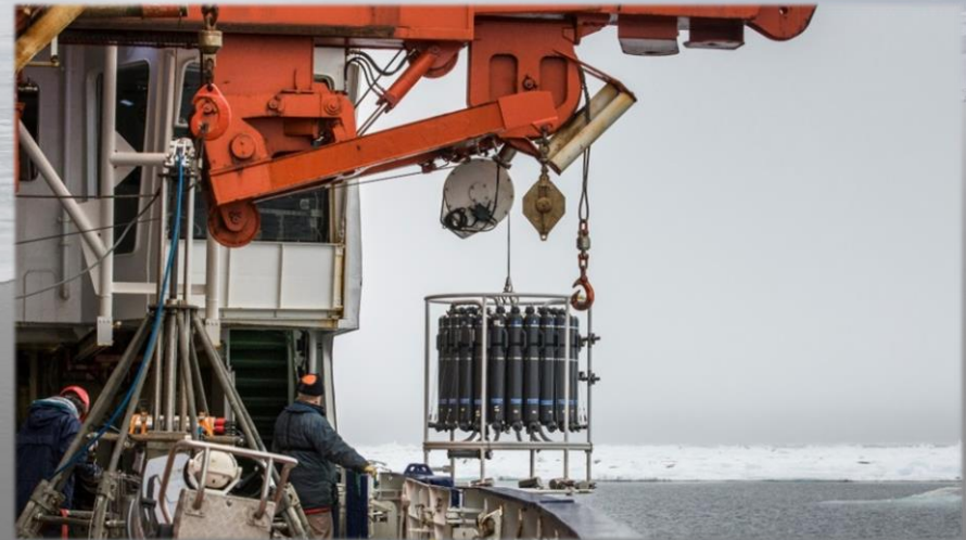
Fig. 11: Water sampling using Niskin bottles rosette.
