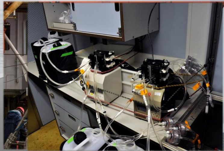
Fig. 12: On board filtration using peristaltic pumps.
