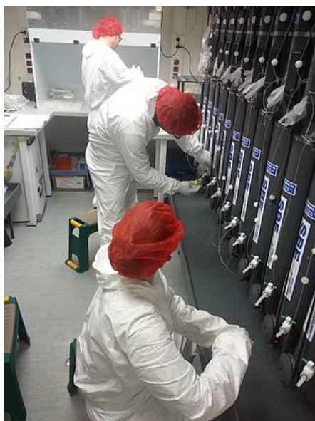
Fig. 1. Bottles with seawater are transferred into a clean room container where the samples are processed under ultra clean conditions for the analysis of trace metals. (Photo: Jaw Chuen Yong)
