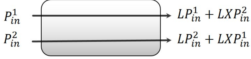
Figure 15: The effect of loss and crosstalk on directional couplers on the input power
