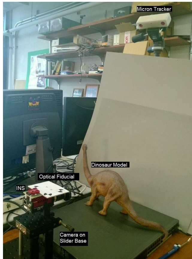
Figure 5-1: Experiment setup for tracking the probe's position relative to the dinosaur phantom.
