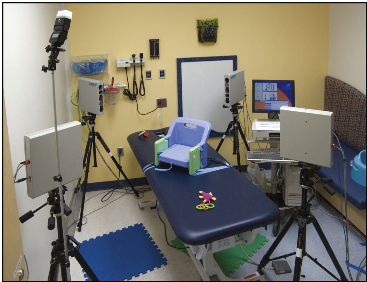
Figure 3 An example of a 3D stereophotogrammetry system (3dMDcranial™ System) in a clinical research setting. The mechanical bed offers a safe surface upon which to secure a booster seat, while allowing the photographer to adjust the participant to ensure an optimal image capture.
