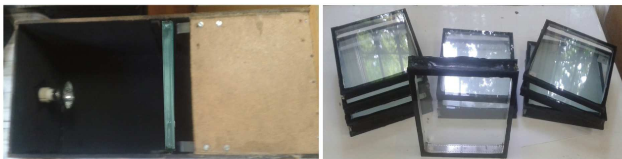
Figure 2. The arrangement of transmittance tests of panels
